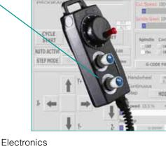
Hand-held Pulse Generator The Rotary hand wheel, attached to the machine, will control the axis that is selected on the wheels dial. All other functions are disabled when this is active.
